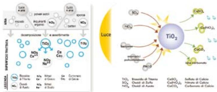
Titanium dioxide is one of the most used catalyst materials, as it has some very specific characteristics which make it very well suited to application on cement and mortar and can immediately be applied as a covering or decoration on walls as well as on previously available surfaces.
